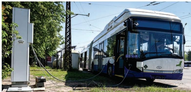
Test refuelling of hydrogen FC range extended trolleybus in Rīga
